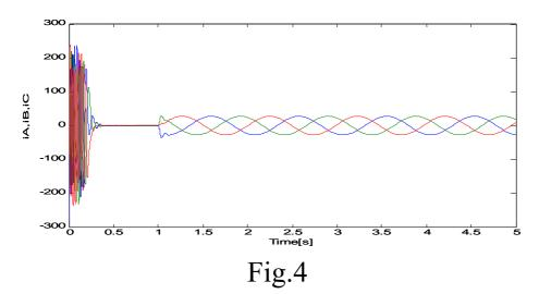
Three phase rotor currents when torque=39[N.m] Starting at no-load motor and at 1sec. torque is enclosed.
