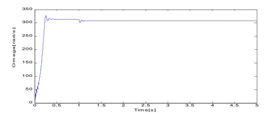
Fig.5 Motor speed when torque=39[N.m]
