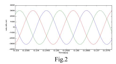
Three phase stator voltages when torque=39[N.m]
