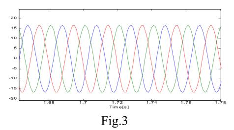
Three phase stator currents when torque=39[N.m]
